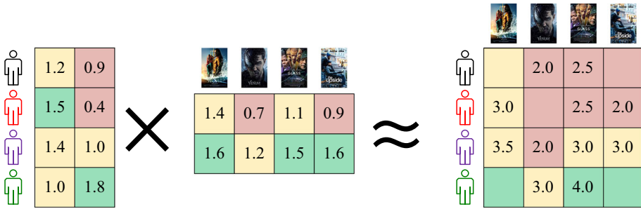
Fig. 2 A simple example for NMF. The incomplete user-item interaction matrix is approximated by the multiplication of two nonnegative matrices, one profiles the user latent features while the other one profiles the item latent features
